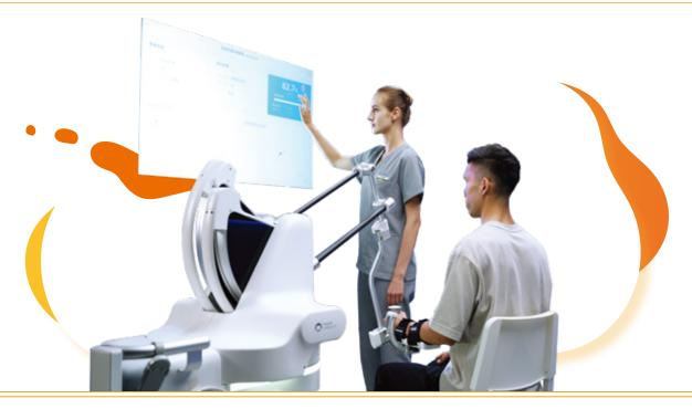
ArmMotus™ EMU is a 3D back-drivable upper limb rehabilitation robot that adopted an innovative cable-driven mechanism, combined with a parallel structure made of lightweight carbon fibre rods which perfectly reduces the friction and inertia of the device. This enables the control system to respond and execute more efficiently, resulting in higher compliance in human-machine interaction.
