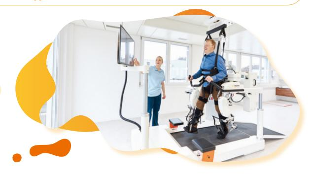
The Lokomat is the world's leading robotic rehabilitation device that provides highly repetitive and the most physiological movement training. This is ensured by the individually adjustable exoskeleton combined with the patented dynamic body weight support system.
