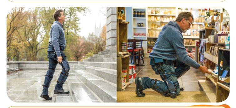
Keeogo<sup>™</sup> is an ambulatory assistive device that is fitted to the lower body, and is powered at the knee. This computer-controlled orthosis provides complementary force to the knee joint throughout a variety of activities, namely:
