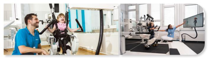
The Lokomat<sup>®</sup> Pro can be fitted with standard orthoses for adults or with Pediatric Orthoses, which are available as an optional add-on module. The Pediatric Orthoses are designed to accommodate small children by offering a special set of harnesses and cuffs that provide a precise fit for patients with femurs between 21 and 35 cm.
