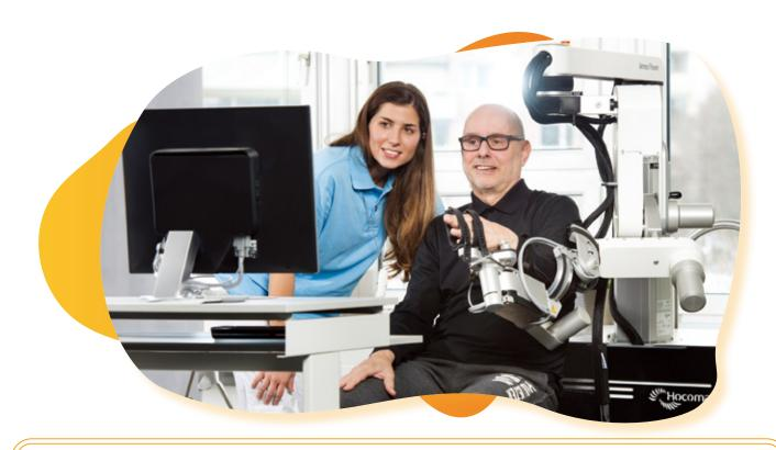
The world's first robotic arm exoskeleton for integrated arm and hand therapy for severely impaired patients. The device enables patients to perform exercises with a high number of repetitions (high intensity), which is paramount for relearning motor function.
