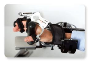
The ManovoSpring is an instrumented hand orthosis to be used as a module in combination with Armeospring for patients with therapy goals focusing on hand rehabilitation.
