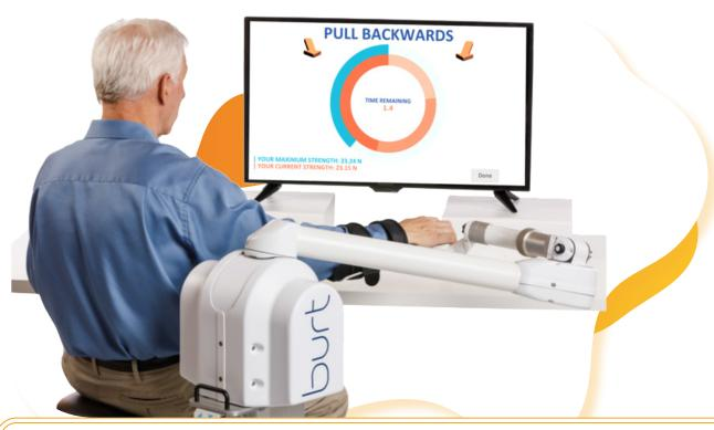
Burt® is an upper-limb therapy robot. It allows a patient to float weightlessly on a cushion of air with GravityCradle™ supporting the patient while applying gentle forces to resist, assist, give subtle queues, and paint a realistic game/activities environment that matches what is visually projected in front of them.
