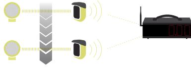
• in combination with the Witty timer; pulses transmitted by the photocells are received by the board and by the timer independently, but in this case, with the timer function, data can be saved and stored for analysis subsequently on a computer using the WittyManager software package
