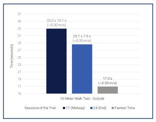
Data from the Indego multi-center study. Figure shows average results of 45 subjects from the 10 Meter Walk Test - Outside. Subjects were tested midway through and at the end of the study. Significant improvements in walking speed have been shown. Highest walking speed measured was 0.59 m/s among all subjects. Subjects continued to improve gait speed through the end of the study even after becoming proficient with the Indego midway through the study.
