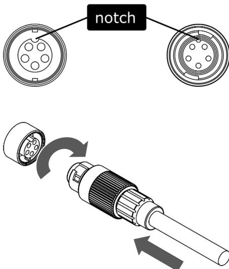
Connect the power supply cable to the power supply socket on the back of the device.
