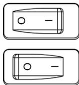
Switch on the Refa by flipping the switch from ‘O’ to ‘I’. On the front panel all LEDs will light up shortly. The Power LED on the front panel will turn green.
