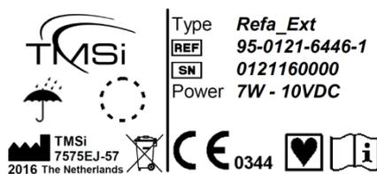
The device label can be found at the bottom of the device (example depicted here, can be different from actual label). It contains the REF code, Serial Number, power requirements and other properties of the device. Use the REF number to look up the channel specifications that can be downloaded from [www.tmsi.com](http://www.tmsi.com).
