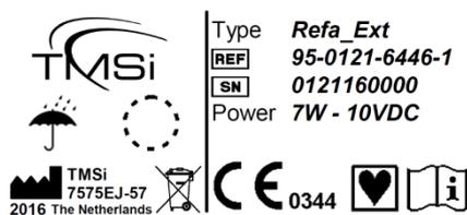
The device label can be found at the bottom of the device (example depicted here, can be different from actual label). It contains the REF code, Serial Number, power requirements and other properties of the device. Use the REF number to look up the channel specifications that can be downloaded from [www.tmsi.com](http://www.tmsi.com).
