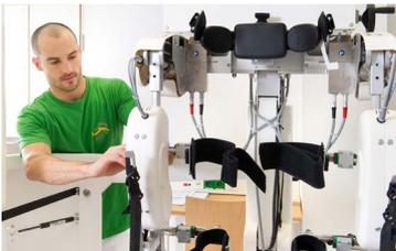
The new FreeD module allowing for lateral and rotational movements of the pelvis. Courtesy of LKH Hochzirl, Austria.
